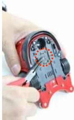
2. Pull out the pin using Long-nose easily
