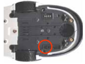
⑥ Turn on the switch on the bottom of the robot.
