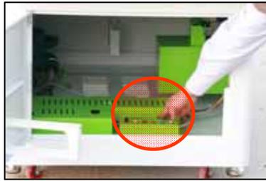
② Turn on the switch on the control box
