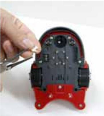
1. Before taking out the pin using Long-nose, cover the pin by cloth or tissue
