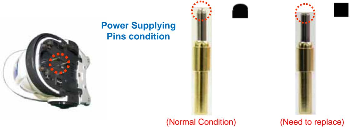
**1) Separation of Power Supplying Pins :** It is easy to take out the pin by pulling it out. If the pin doesn't pull out by hand, use a long-nose to take out . At this point, use cloth or tissue to cover the pin to protect, then use a long-nose to pull out
